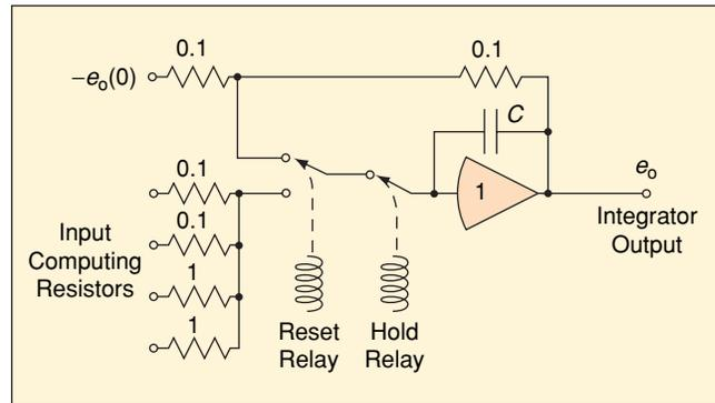
**Figure 3.** Circuit for integrator mode control. The reset relay, when energized, establishes the initial condition for the integrator. The hold relay, when energized, stops the integration and freezes the output voltage  $e_o$ .
