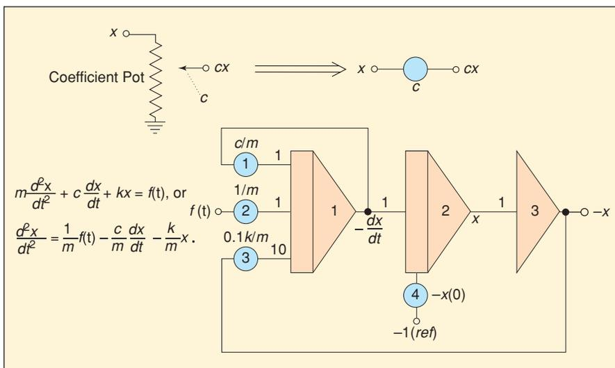
**Figure 7.** Using potentiometers to set coefficient values in an analog simulation circuit. Note that pot 3 is set at  $0.1 c/m$  because of the gain-of-10 input. To speed up the setting of coefficients in large problems, servo-set potentiometers were widely used in state-of-the-art analog computers.
