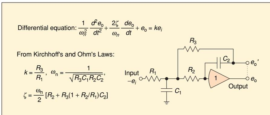
**Figure 6.** Single-amplifier circuit for simulating a second-order system when  $e_o' = e_o$ . For the closed-loop system to be stable with a phase margin of  $\pi/2$ , the open-loop frequency response should exhibit a slope of  $-6$  dB/octave at and around the frequency of unity (0 dB) open-loop gain.
