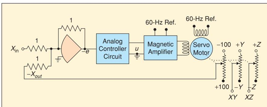
**Figure 8.** A servomultiplier that uses a 60-Hz, two-phase servo motor driven by a magnetic amplifier. The analog controller circuit is used to provide additional damping. Typical multiplier accuracy was 0.1% or better. Because of the limited servo bandwidth, the servo input  $X_{in}$  should be assigned to the slower of the two variables in computing a product.
