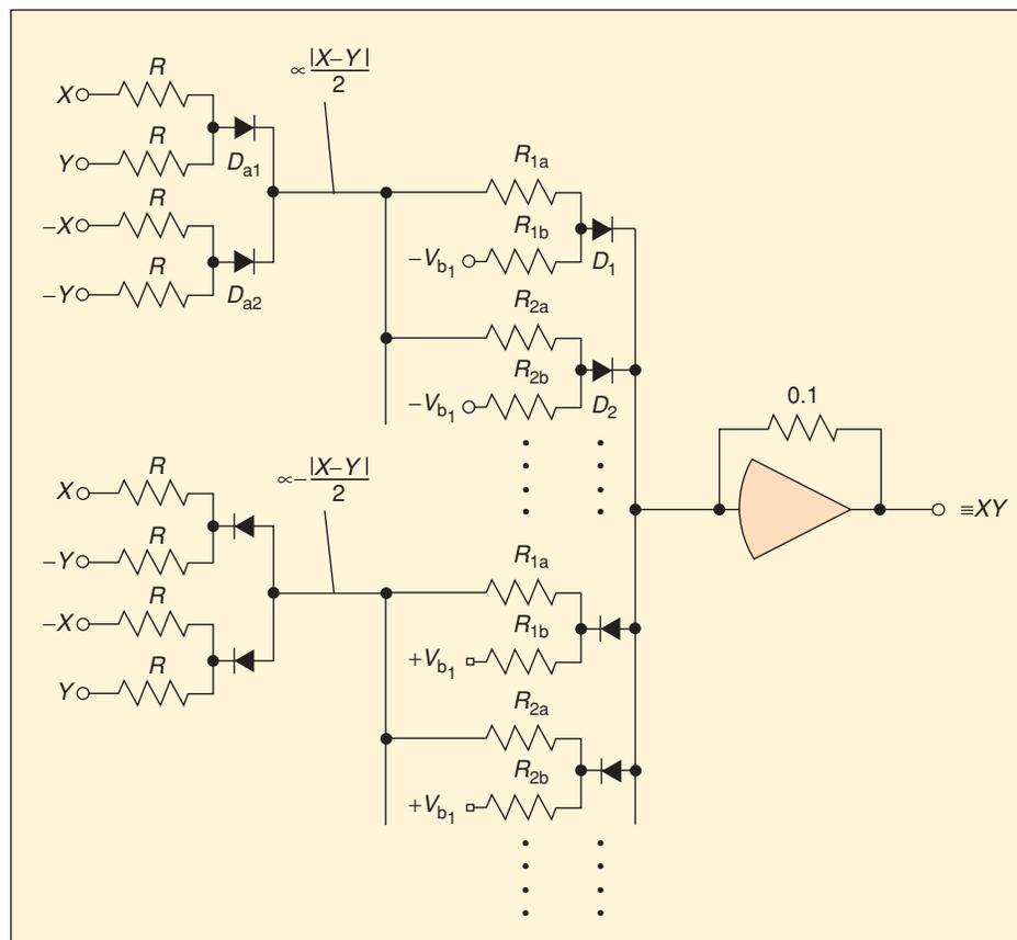
**Figure 11.** A completely passive quarter-square multiplier circuit terminated in a single operational amplifier. The circuit is based on  $XY = (|X + Y|/2)^2 - (|X - Y|/2)^2$ . The circuit output is connected to the summing junction of an operational amplifier with a 0.1 mΩ feedback resistor.
