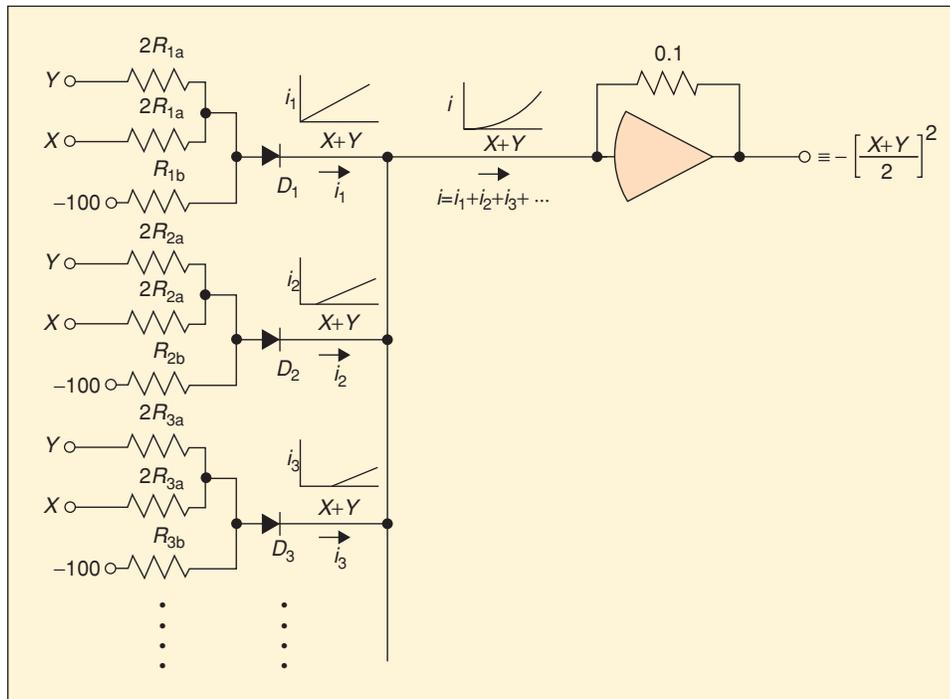
**Figure 10.** Diode circuit for approximating  $((X + Y)/2)^2$  for  $X + Y > 0$ . The same circuit is repeated with inputs  $-X$  and  $-Y$  to approximate  $((X + Y)/2)^2$  for  $X + Y < 0$ . A similar pair of circuits with inputs  $X$  and  $-Y$ , and  $-X$  and  $Y$ , with diodes reversed and  $+100$  bias voltages, is used to approximate  $-((X - Y)/2)^2$ . A single operational amplifier is used to sum the outputs of all four circuits to produce the product  $XY$ .
