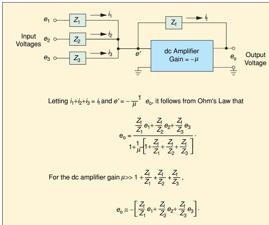
**Figure 1.** Operational amplifier. When the feedback and input impedances are resistors, the output voltage is proportional to the sum of the input voltages. When a capacitor  $C$  is used as a feedback impedance,  $Z_f = 1/(Cs)$  and the output voltage is proportional to the time integral of the sum of the input voltages.
