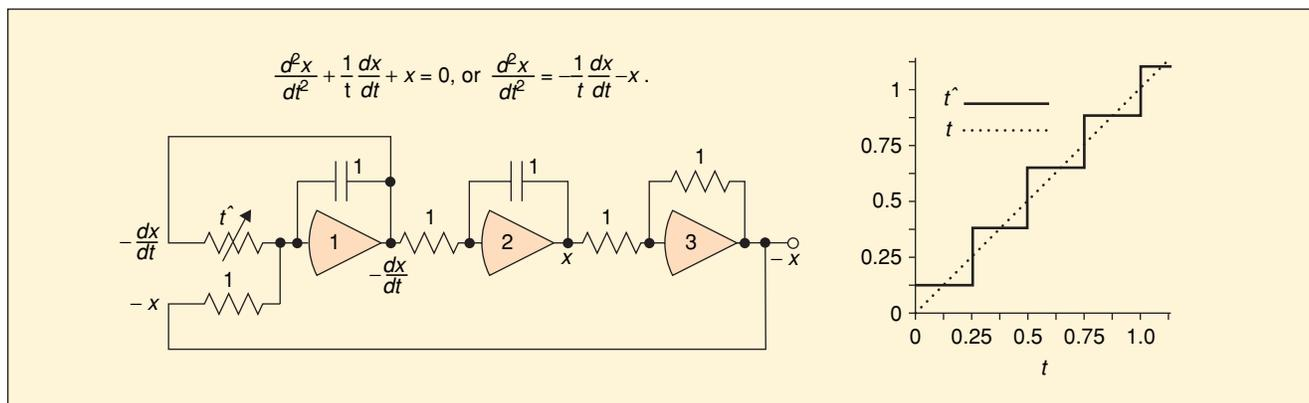
**Figure 4.** Analog circuit for solving Bessel's equation of order zero. The variable coefficient is approximated with the staircase function using a stepping relay.
