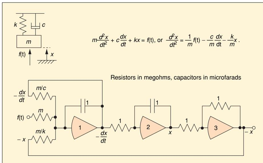
**Figure 2.** Analog circuit for simulating a mass-spring-damper system. Amplifier 1 sums the terms in the equation for  $d^2x/dt^2$  and integrates the sum to obtain  $-dx/dt$ . Amplifier 2 integrates  $-dx/dt$  to obtain  $x$ . Amplifier 3 simply inverts  $x$  to obtain  $-x$ . Note that all integrators are inverting.
