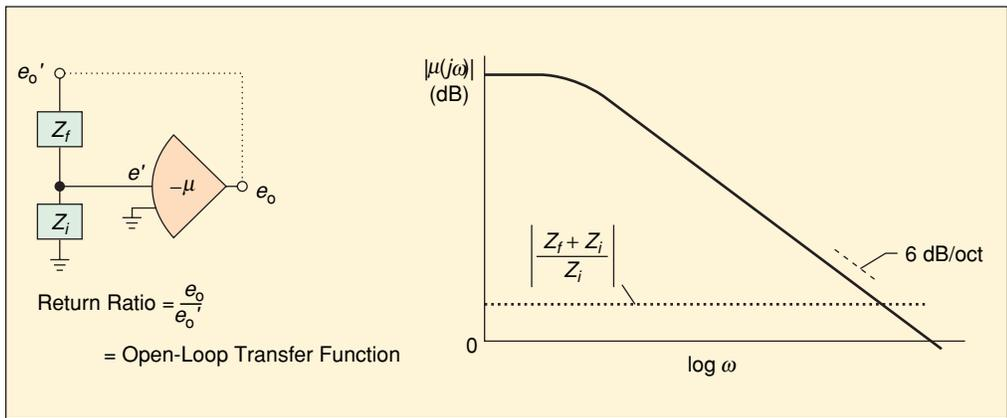
**Figure 5.** Operational amplifier frequency response. This open-loop frequency response is needed to provide 90° of phase margin for any ratio of feedback to input impedances.
