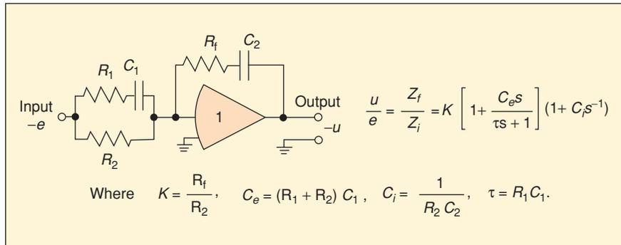
**Figure 9.** One-amplifier analog controller circuit for proportional, bandwidth-limited rate and integral control. Alternatively, a circuit that requires two conventional integrating amplifiers and two summing amplifiers can be used.
